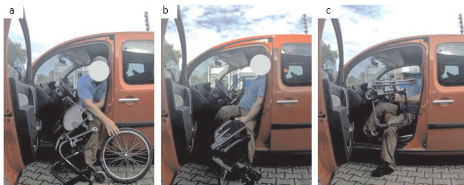
Fig. 7. Differences when entering the vehicle in the way the wheels are arranged when detaching them: a – wheels placed on the side of the vehicle (M2in), b – wheels placed on the front right seat (M3in), c – wheel detached inside the vehicle (M4in)
