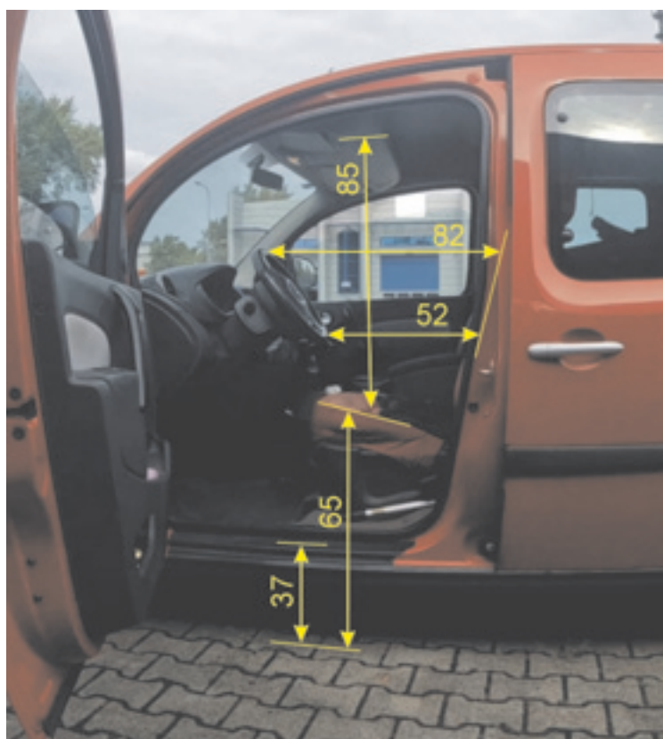
Fig. 3. Key dimensions in centimeters of the vehicle access space
